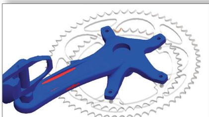
Estimate component life based on calculated or SolidWorks Motion loads.
