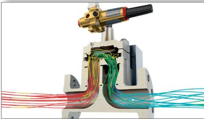
Examine complex flow in and around components to detect turbulence and recirculation issues and determine flow conditions.
